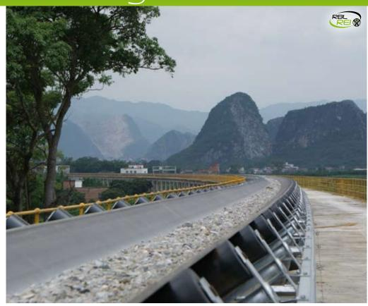
RBL-REI is currently delivering two 40km lines of conveyor belt in FENG-KAI (China). These two parallel lines, each at 2,500 t/hr, will supply one of the world's largest cement works with 30,000 tons of cement a day. Each line includes 3 Curvoduc™ (11, 12 and 17km), powered in total by nineteen 750 kW driving units, with a belt speed of 5 m/s. Curved conveyors (Curvoduc™) are suitable for
